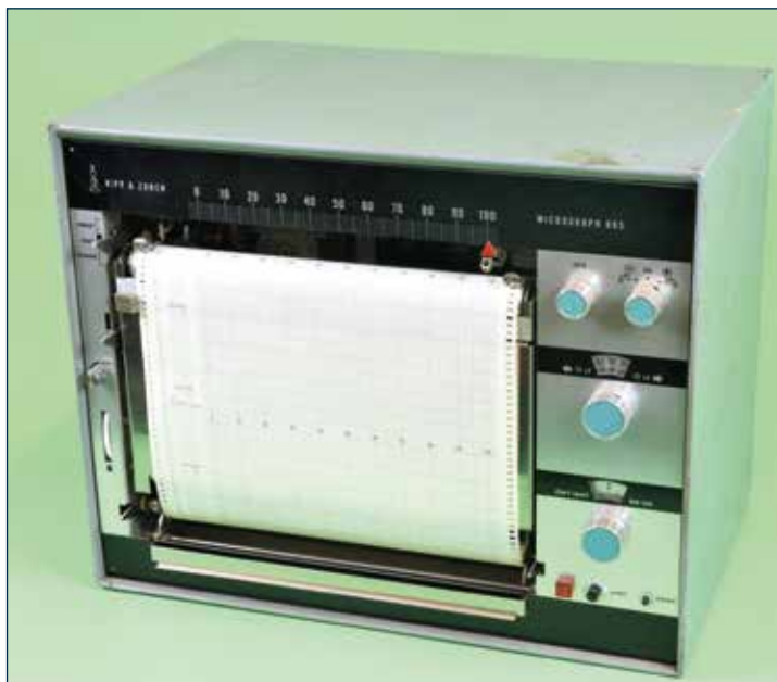
Fig. 7 BD5 - First recorder with semiconductor input 1968 – V32128.
