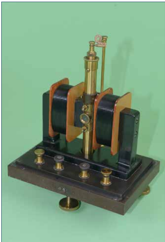
Fig. 1 Moll coil mirror galvanometer 1913 - V06652.
